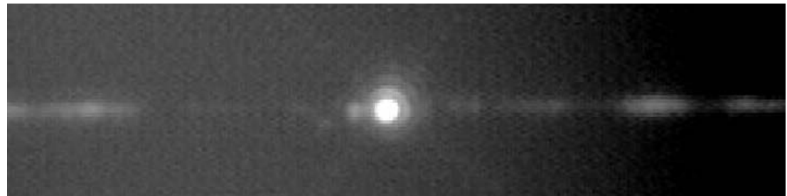
1550 nm light transmitted through the nanowire waveguide with tapered coupler
